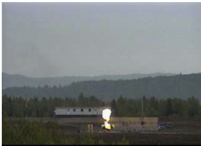
Fig. 2. Failure of 2000 L ASME code propane tank (two-phase jet release continues, t = 17 ms).
