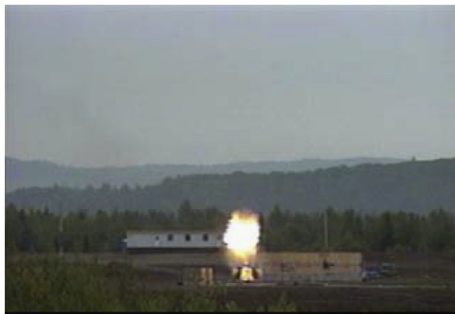
Fig. 3. Failure of 2000 L ASME code propane tank (two-phase jet release continues, fracture growing rapidly, t = 34 ms).
