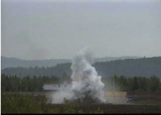
Fig. 5. Failure of a 2000 L ASME code propane tank (shock is visible and overtakes cloud release, t = 67 ms).
