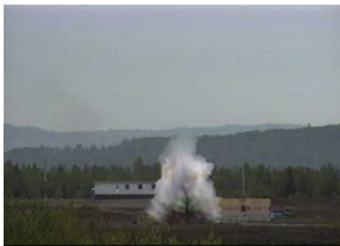
Fig. 4. Failure of 2000 L ASME code propane tank (wall fails catastrophically with BLEVE, shock and cloud coincident, t = 50 ms).
