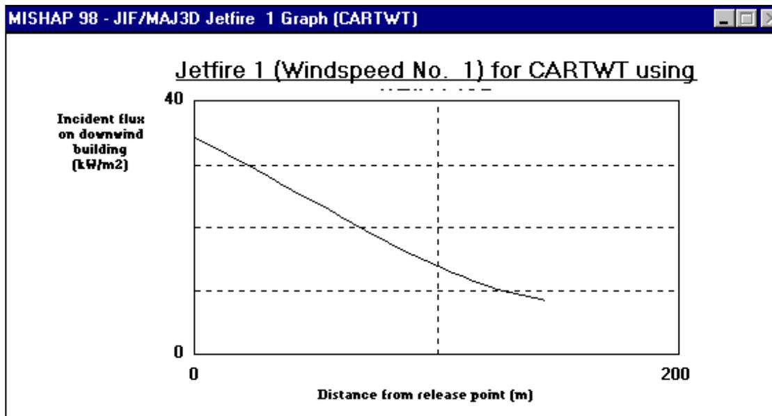
Figure 3 Graph of Flux versus distance downwind
