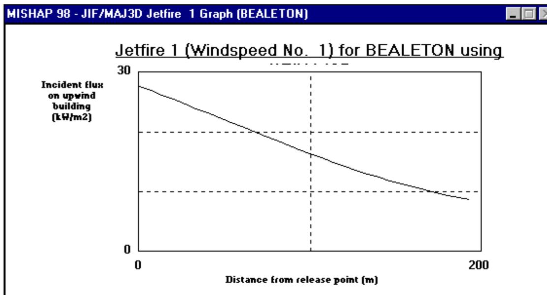
Figure 5 Graph of Flux versus distance
