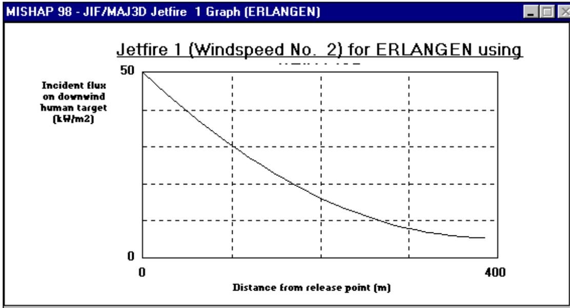
Figure 4 Graph of Flux versus distance
