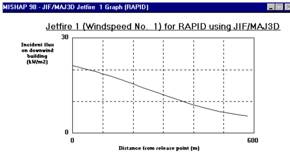
Figure 6 Graph of Flux versus distance
