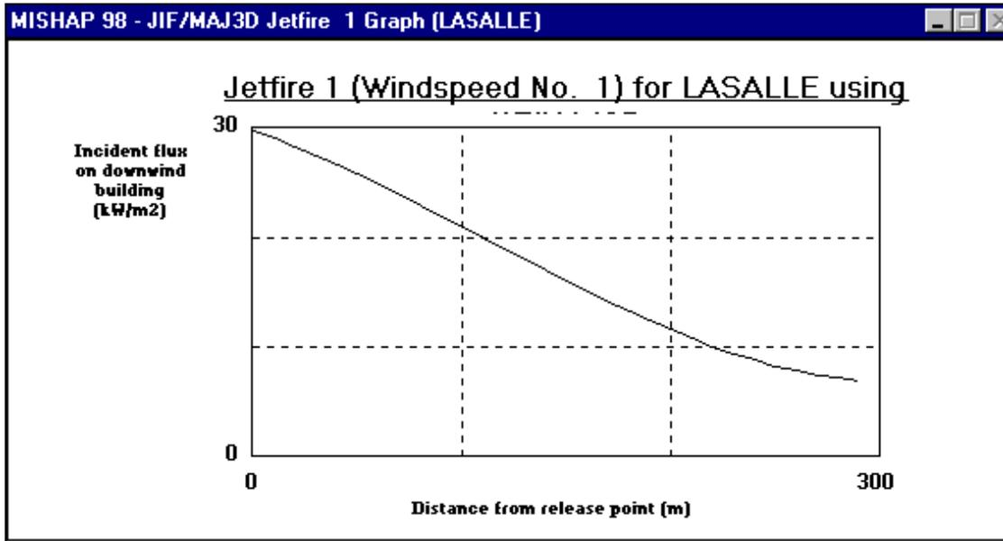
Figure 4 Graph of Flux versus distance
