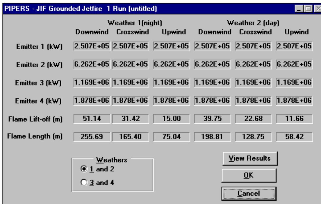
Figure 4 Results from PIPERS for a Grounded Jet
