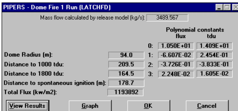
Figure 6 Results from a dome fire model
