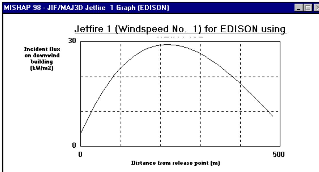
Figure 7 Flux under the axis of a Tilted Jet-fire 10m above Ground Level
