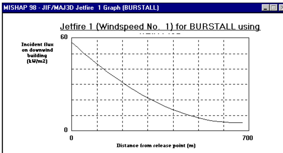
Figure 5 Graph of Flux versus distance downwind
