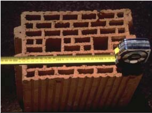
Figure 3-10 Hollow clay tile block used for infills
