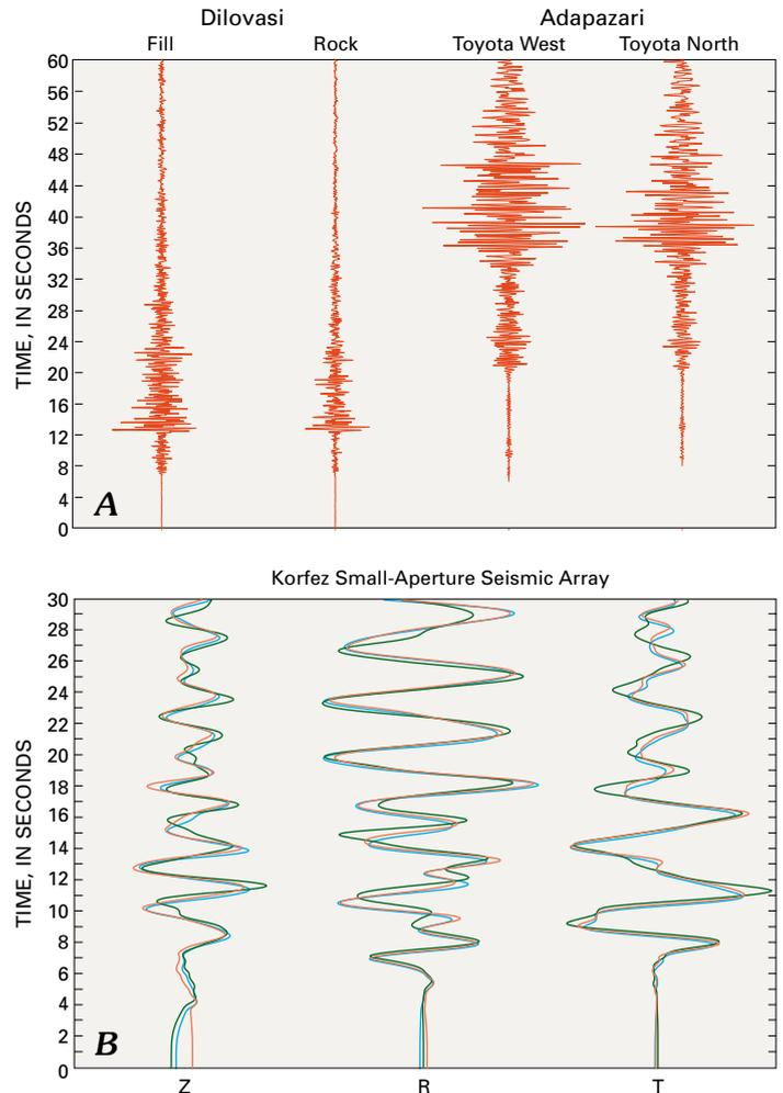
**Figure 32.** A, Pseudo-record section of ground motions from two pairs of stations at Dilovasi and Adapazari plotted on the same amplitude and time scales. Note the S-minus-P time of the first pair is approximately 5 s and that of the second is approximately 16 s. B, Overlay of Z, R, T components of closely spaced North, South, West stations at Korfez, all traces plotted on the same amplitude and time scales. *Illustration by Edward Cranswick.*
