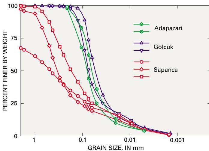
**Figure 39.** Grain-sized distributions of sand boils sampled near sites of sunken buildings in Adapazari, Gölcük, and Sapanca. Vertical axis is percent of sample by weight finer than the grain size shown on the horizontal axis. *Illustration prepared by Michael J. Bennett. Data from USGS and ERDC.*
