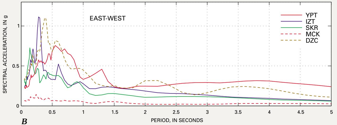
**Figure 26.** Actual pseudo-acceleration response spectra (**A**, **B**) and normalized (with respect to zero-period acceleration) response spectra (**C**, **D**) for 5 stations. The normalized response spectra also show the response spectra of the 1998 Turkish Building Code for stiff and alluvial soil site conditions. *Illustration by Mehmet Çelebi.*
