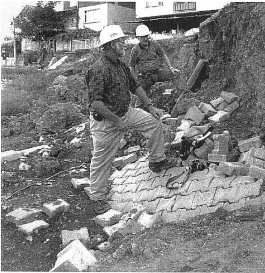
Figure 2 - Fault scarp east of Golcuk. The vertical displacement is 2.3 m down-to-the north, with 1.3 m of right slip. (Photo: Mark Milstein, Atlantic News Service)
