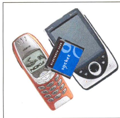
Figure 7.1.37. Hardware required to gather digital damage building data, a hand computer and cellular phone having bluetooth interface
